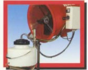
Wanjet F22 & F23 have a agitation system, working by an electric motor, which is assembled on a telescope arm.
